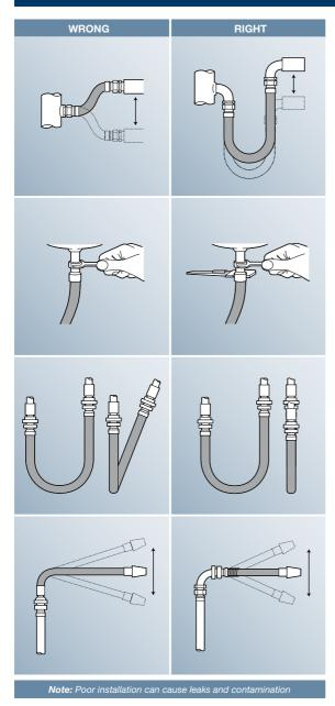
Flexible Hose Assemblies (FHA's) should always be handled with reasonable care, and should not be subjected to over straining. The design of hose supports and saddles should be to ensure that the minimum bend radius is not compromised.
